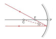
**Rule 3**: If an incident ray passes through the centre of curvature of the mirror, then the reflected ray traces the same path back.
