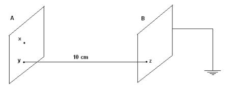
A is given a positive potential of 10 V, and the other surface of B is earthed.
