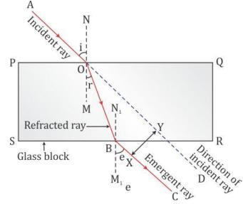
From the figure, we can see that the incident ray is parallel to the emergent ray but with a lateral displacement.
