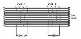
Two coils of insulated copper wire are wrapped on few long iron rods. Coil-1 is connected to a battery through a switch and Coil-2 is connected to a galvanometer. Now, the current is switched on in Coil-1. A momentary deflection is seen in the galvanometer attached to Coil-2. The deflection is due to current induced in Coil-2 momentarily as the magnetic field builds up along the axis of Coil-1 when current is switched on.
