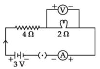
Find the reading of (i) the ammeter and (ii) the voltmeter.
