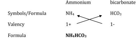
Therefore, the molecular formula of Ammonium bicarbonate is NH4HCO3
