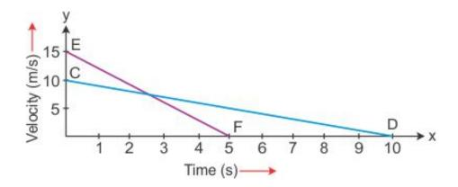
Distance travelled by A = Area under EF =  $\frac{1}{2} \times 15 \times 5 = 37.5$  m
