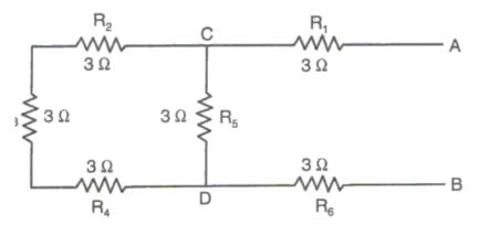
For the combination of resistors shown in the figure, find the equivalent resistance between (i) C and D (ii) A and B.
