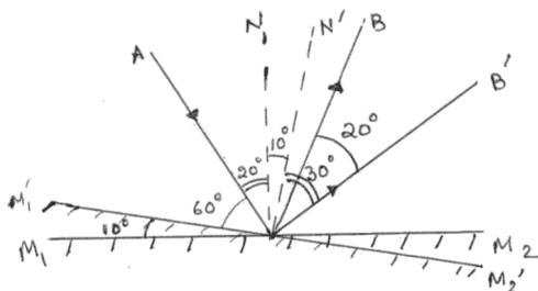
Angle between incident ray and final reflected ray =  $30^\circ + 30^\circ = 60^\circ$
