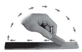
Now, take a bar magnet and place one of its poles near one edge of the bar of iron.
