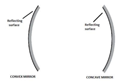
• Spherical mirrors are obtained by slicing a section from a hollow sphere.
